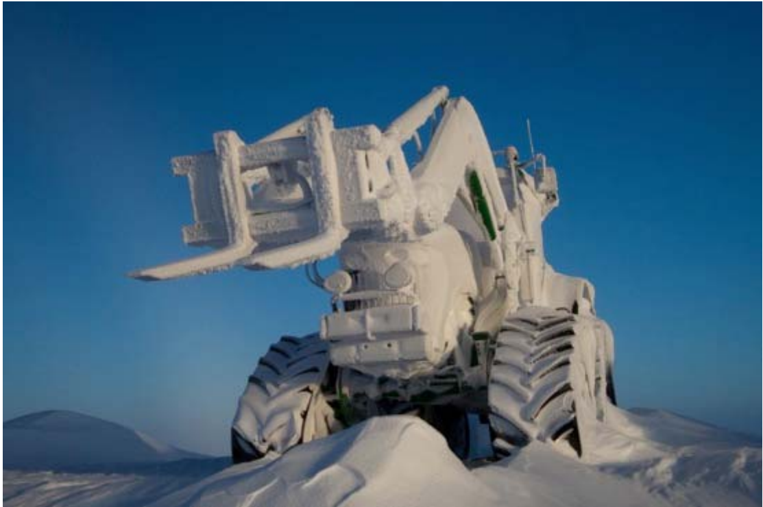
Photo 19: The state the vehicles were in each day following the extreme cold weather. It would often take days to 'de-frost' vehicles when they were in this condition before they could be used again
